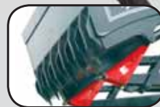
Teeth on top and bottom overlap and close tightly to handle loose materials. When open, it acts as a dozer blade to pack silage or move snow.
