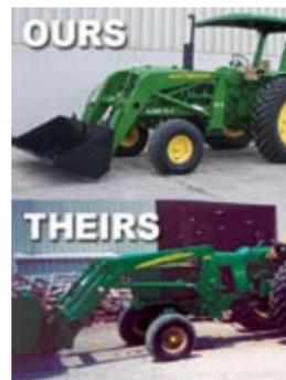
front tires; as a result, placing it on a 2WD tractor will require the loader to sit farther forward and higher along the hood.
