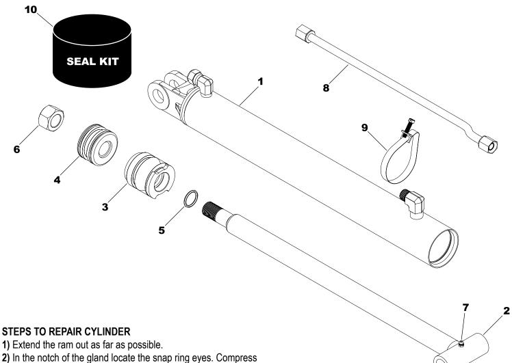
the snap ring with a snap ring pliers.
